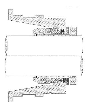
NOTE: Make sure the stuffing box locknut is on the shaft **PRIOR** to placing pump case into position. This nut is used to tighten the seal into place.
